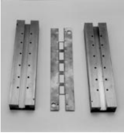
Fig. 11. Photograph of the E-plane bandpass filter with improved stopband performance.
